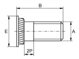
For plate thickness, min = 1.5 Head diameter E = 6 Hole diameter +0.1 = 4.2 Length B = 15 Male thread A = M3x0,5 Min distance to edge = 2.4
